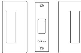
Passage handles are suitable for situations where locking or latching is not required. These handles do not have a striker or magnet.
