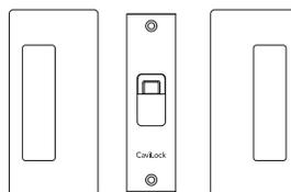
The Bi-Parting mate includes a striker on the face plate to enable it to latch with a privacy handle. For Bi-Parting passage doors, order two single passage handles.
