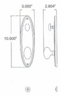
5360-XXX-ENTR 5360-XXX-DBLC 5360-XXX-FD Single Cylinder Entrance Set - adjustable backset latch and deadbolt 2-3/8" & 2-3/4" Double Cylinder Entrance Set - adjustable backset latch and deadbolt 2-3/8" & 2-3/4" Full Dummy Set 6.76 lbs. 6.98 lbs. 5.10 lbs.
