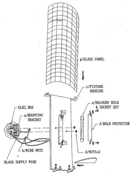
FIT THE BOTTOM GLASS TO THE FIXTURE HOUSING (c) AND SECURE WITH BRASS SCREWS (ATTACHED) GENTLY.
