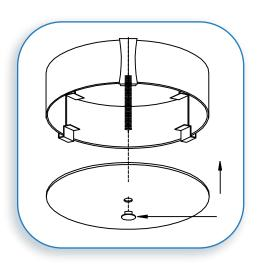
**COVER THE FLAT GLASS** Fit the flat glass to the base of the curved glass
