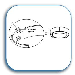
Take the 3pcs curved glass and align them so that they slide in, from opposite sides, into the middle of the metal brackets. Align the holes in the glass with the holes in the metal brackets. Using the glass security screws tighten so that glass security screws are flush to the metal brackets.
