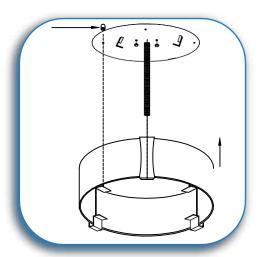
**SECURE THE ROUND METAL PLATE** Align the holes on the metal brackets and
