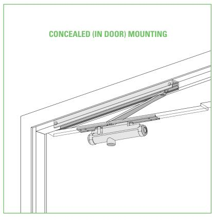
The concealed 3130 is designed to mount in a 1 3/4" interior door. The single lever arm and roller assembly provides complete concealment and the choice of finishes and track functions meet virtually all architectural requirements.
