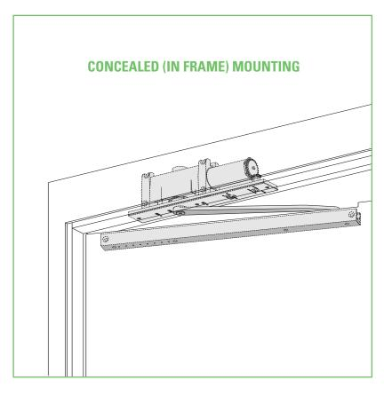
The concealed 2010 Series is a heavy duty closer designed to provide complete concealment.
