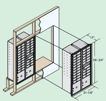
Note: For U.S.P.S. serviced installations, the tenant locks in the top row of mailboxes must be no more than 67" above the finished floor and the bottom shelf of the lowest row of mailboxes must be no less than 28" above the finished floor. The U.S.P.S. master arrow lock must be a minimum of 36" and a maximum of 48" above the finished floor. The bottom shelf of parcel lockers must be at least 15" above the finished floor.
