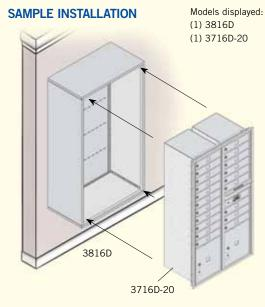
Note: For U.S.P.S. serviced installations, the tenant locks in the top row of mailboxes must be no more than 67" above the finished floor and the bottom shelf of the lowest row of mailboxes must be no less than 28" above the finished floor. The U.S.P.S. master arrow lock must be a minimum of 36" and a maximum of 48" above the finished floor. The bottom shelf of parcel lockers must be at least 15" above the finished floor.
