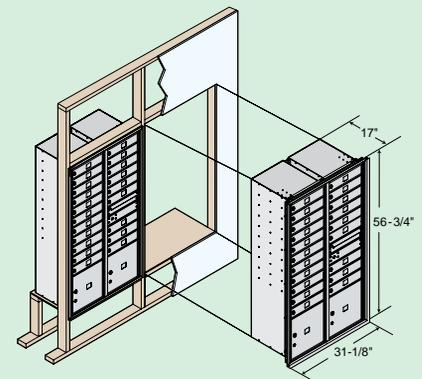
*Note: For U.S.P.S. serviced installations, the tenant locks in the top row of mailboxes must be no more than 67" above the finished floor and the bottom shelf of the lowest row of mailboxes must be no less than 28" above the finished floor. The U.S.P.S. master arrow lock must be a minimum of 36" and a maximum of 48" above the finished floor. The bottom shelf of parcel lockers must be at least 15" above the finished floor.*
