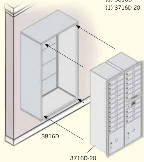
*Note: For U.S.P.S. serviced installations, the tenant locks in the top row of mailboxes must be no more than 67" above the finished floor and the bottom shelf of the lowest row of mailboxes must be no less than 28" above the finished floor. The U.S.P.S. master arrow lock must be a minimum of 36" and a maximum of 48" above the finished floor. The bottom shelf of parcel lockers must be at least 15" above the finished floor.*
