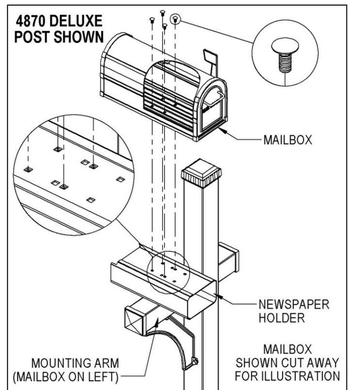
Note: On the 4870 deluxe mailbox post, the longer mounting arm which accommodates the newspaper holder and mailbox can be on either the left or right side. When attaching the post to the ground, position the post so the longer mounting arm is on the side desired. Then mount the newspaper holder and mailbox on the mounting arm with the mailbox facing the street or roadway.
