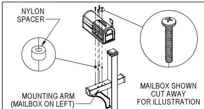
Note: On the 4870 deluxe mailbox post, the longer mounting arm which accommodates the mailbox can be on either the left or right side. When attaching the post to the ground, position the post so the longer mounting arm is on the side desired. Then mount the mailbox on the mounting arm with the mailbox facing the street or roadway.
