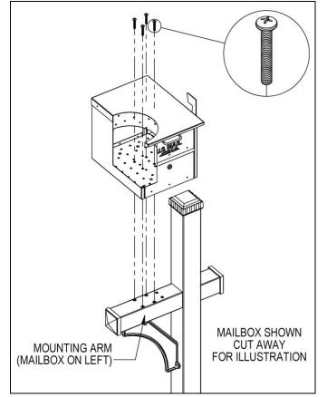
Note: On the 4370 deluxe mailbox post, the longer mounting arm which accommodates the mailbox can be on either the left or right side. When attaching the post to the ground, position the post so the longer mounting arm is on the side desired. Then mount the mailbox on the mounting arm with the mailbox facing the street or roadway.
