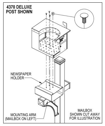
Note: On the 4370 deluxe mailbox post, the longer mounting arm which accommodates the newspaper holder and mailbox can be on either the left or right side. When attaching the post to the ground, position the post so the longer mounting arm is on the side desired. Then mount the newspaper holder and mailbox on the mounting arm with the mailbox facing the street or roadway.
