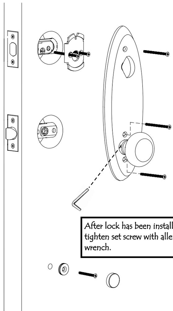
After lock has been installed tighten set screw with allen wrench.
