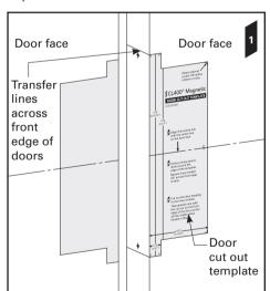
**2.** Mark two holes in the centre of the door thickness in the positions shown. Using these marks, drill two 2.5mm (3/32") diameter holes to a depth of 35mm (1-3/8").
