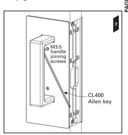
**8**. Fit the *Bi-Parting face plate* to the chassis using the 3x *face plate screws*.
