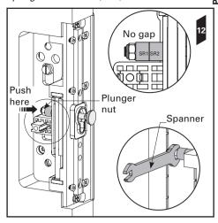
13. Two identical spanners have been supplied. Restrain the plunger nut using the large end of one of the supplied spanners. Place the small end of the second spanner across the flats under the head of the plunger. Keep the spanner restraining the plunger nut stationary while turning the second spanner clockwise.
