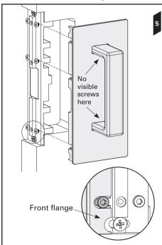
**6.** Fit the remaining Bi-Parting side handle to the chassis and tighten the 3x side handle to chassis screws.
