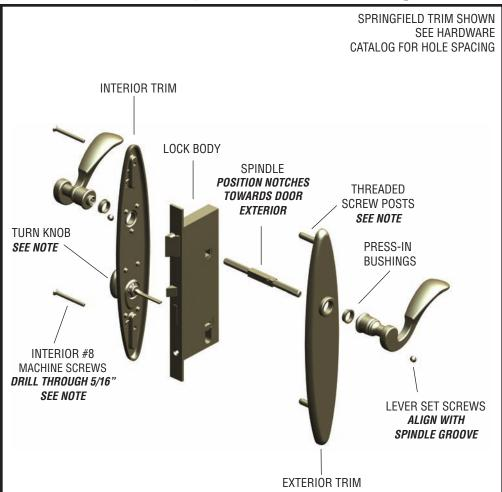
**Turn Knob Note:** Shown is the lever on the top of the turn knob. The lever may be on the bottom, depending on the lock.
