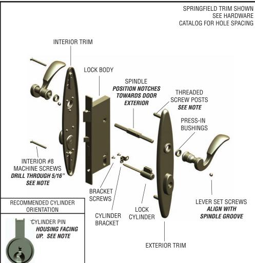
Lock Cylinder Note: Shown is the lever on the top of the lock cylinder. The lever may be on the bottom, depending on the lock.
